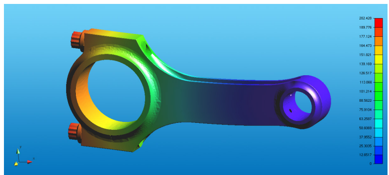
This connector rod was modeled in Cobalt (top) and brought into Iridium for meshing and analysis. The visualizations in Iridium show (middle) the von Mises stress analysis, and (bottom) the displacement.
