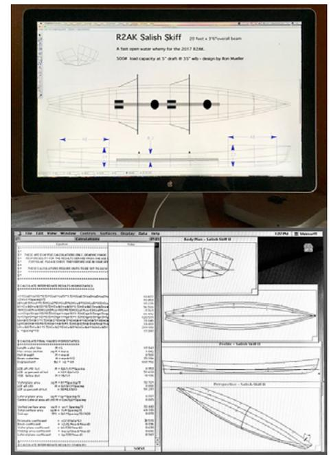
Using specialty hull design software, Mueller then exported a DXF file and brought it into Graphite to designate equipment placement and layout buildable lengths, nested together on 4'x8' sheets of plywood to be cut by his CNC machine.
